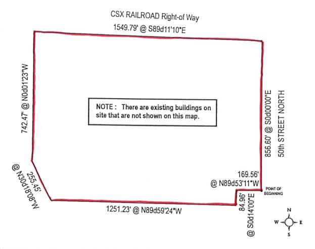
Commence at the SE corner of Section 17, Township 17 South, Range 2 West and run west along the south line of said section 25.01 feet to the intersection with the west right-of way line of 50th Street North; thence turn right and run N0d00'00"W along said right-of way line 446.05 feet to the POINT OF BEGINNING;
